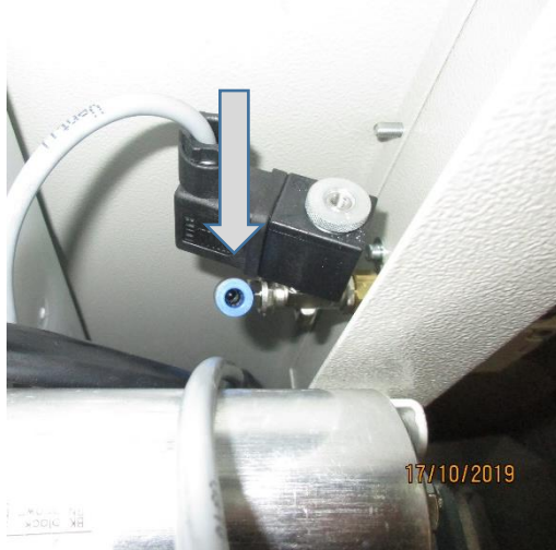
Fig. 2: Pneumatic air supply for actuating the ratchet cylinders.
