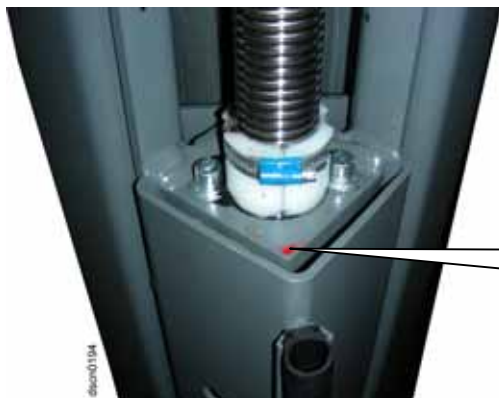
pic 16: the carrying-nut wear pin marked with red safety colour
