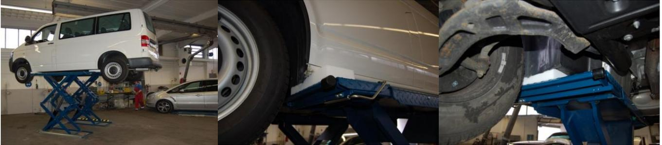
Safety lifting at the original and required pick-up points from car's manufacturers:
